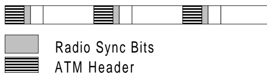
Figure 5 – Radio Frame Structure
