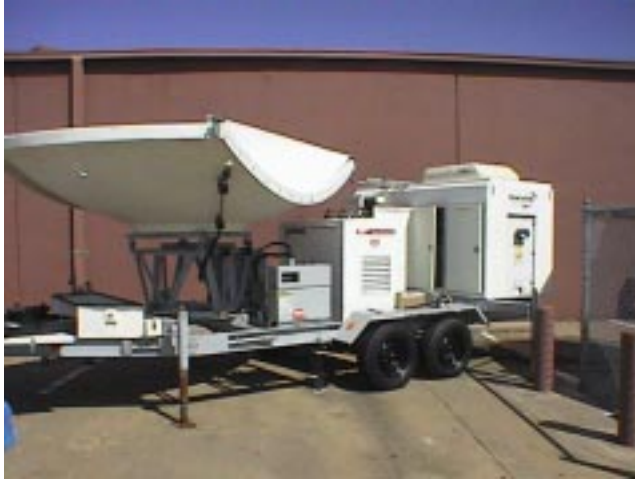
Figure 2: Transportable Earth Station (Trailer-Mounted)
